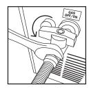
2 Ensure gas line is connected properly
