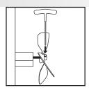
4 Remove fan blade with 3/32 T-handle Allen wrench
