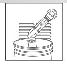
8 Drain grease into approved container using flex hose
