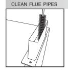
Insert flue brush all the way down to handle to remove build up
