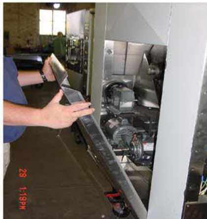
Step 8 - Remove Convection System Access Panel. Carefully Lift Out & Lift Up.
