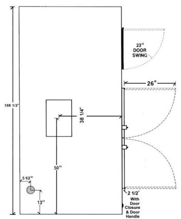
**Construction:** Heavy duty 12 gauge steel interior side walls (100% welded & inspected seams) tubular steel frame, 22 gauge stainless steel exterior, mineral wool insulation – rated 1200 degrees F. (contains no asbestos or fiberglass)
