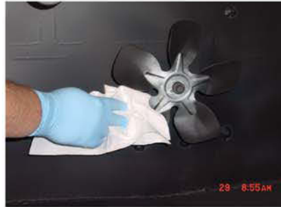
Step 5 - Clean the Fan Assembly(s) Completely. Check for Signs of Imbalance or Irregularities.
