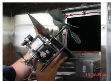
Step 7 - Slowly Remove the Convection Fan Assembly(s).
