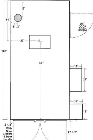
**Construction:** Heavy duty 12 gauge steel interior side walls (100% welded & inspected seams) tubular steel frame, 22 gauge stainless steel exterior, mineral wool insulation – rated 1200 degrees F. (contains no asbestos or fiberglass)
