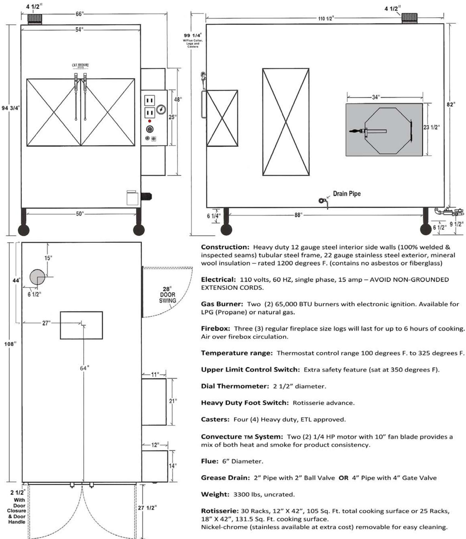
**Construction:** Heavy duty 12 gauge steel interior side walls (100% welded & inspected seams) tubular steel frame, 22 gauge stainless steel exterior, mineral wool insulation – rated 1200 degrees F. (contains no asbestos or fiberglass)
