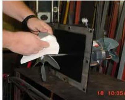
**Step 8. - Clean Fan Assembly(s) Completely. Check
