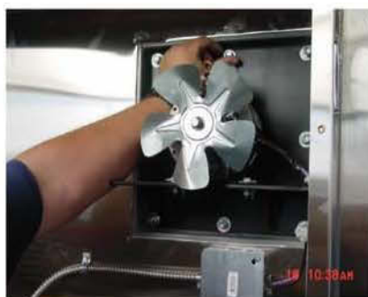
Step 5 - Remove Nuts, Lock Washers & Washers.
