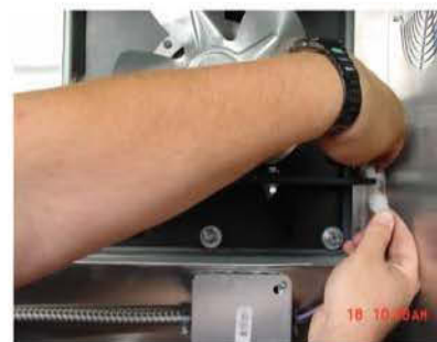
Step 3 - Unplug the Quick Disconnect.
