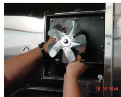
Step 6 - Place a Firm Hold on the Motor Mount & Motor...
