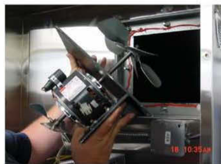
Step 7 - Slowly Remove the Convection Fan Assembly(s).
