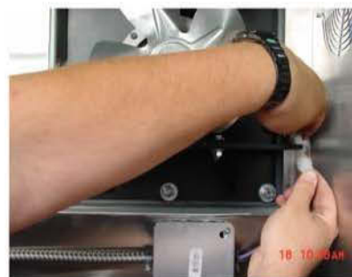
Step 3 - Unplug the Quick Disconnect.
