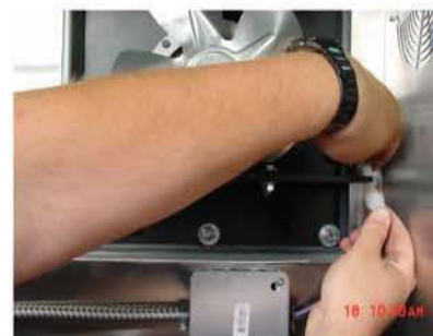
Step 3 - Unplug the Quick Disconnect.
