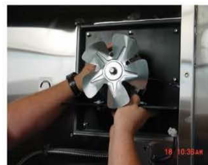
Step 6 - Place a Firm Hold on the Motor Mount & Motor...
