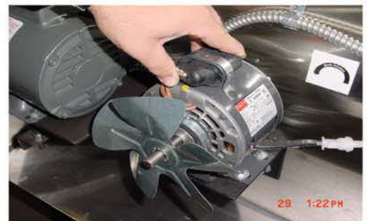
Step 9 - Clean Fan Blades as needed and check for Signs of Imbalance or Irregularities.
