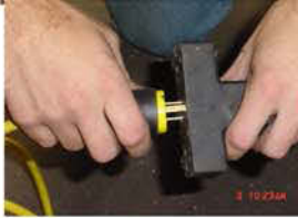
Step 1 - Turn Off & Unplug Unit Before You Start.
