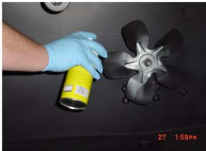
Step 4 - Spray Both Sides of Fans with Degreaser/Cleaner.
