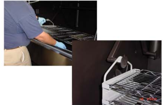
Step 6 - Reinstall the Rack Configurations, so that they Rest Correctly on the Trunion.
