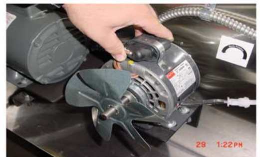
Step 9 - Clean Fan Blades as needed and check for Signs of Imblance or Irregularities.
