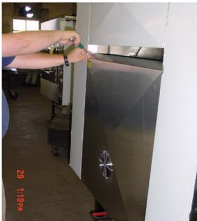
Step 7 - Remove Screws to Convection System Access Panel.
