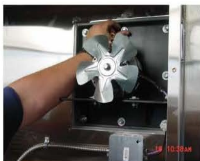
Step 5 - Remove Nuts, Lock Washers & Washers.
