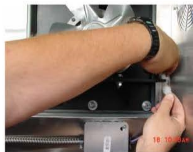
Step 3 - Unplug the Quick Disconnect.
