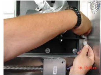
Step 3 - Unplug the Quick Disconnect.
