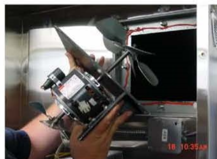
Step 7 - Slowly Remove the Convection Fan Assembly(s).
