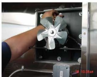
Step 5 - Remove Nuts, Lock Washers & Washers.
