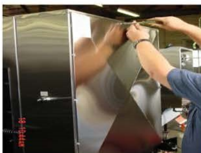
Step 2 - Remove Service Panel Located at the Back of the Unit.
